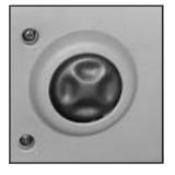
If your vehicle has power lumbar adjustment, you can use it to increase or decrease lumbar support in the lower seatback. The control is located on the outboard side of the seat cushion.
